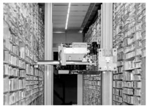
typical range of articles in this sector. The automatic picking solution includes an articulated arm robot with a flexible gripper, precise image recognition and processing, specialized control software and a comprehensive safety concept.
